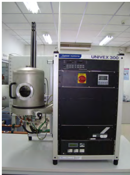
Figure 4.6 Metal evaporator Equipment.
