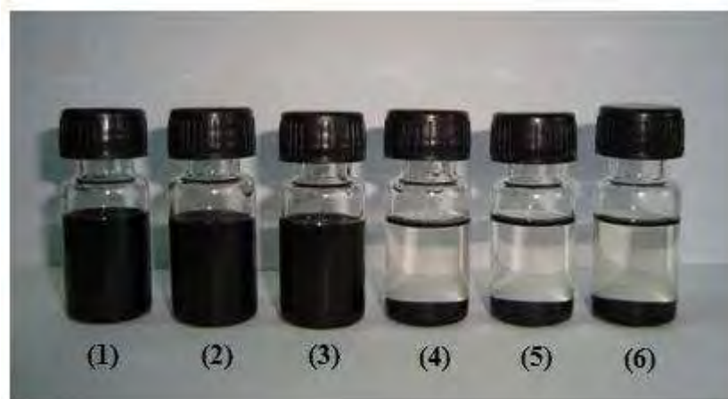
Figure 5.3 Vials (6mL) containing the CB suspension (0.15 wt/v%), in which the CB to SDS ratio were 1:0.4 (1), 1:0.8 (2) and 1:2 (3) sample were imaged after sonication 3 months whereas 1:5 (4), 1:10 (5) and 1:100 (6) sample were imaged after sonication 36-48 hours.
