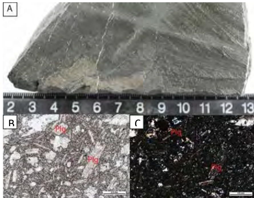
Fig. 4.12 Characteristics of plagioclase phyric andesite, (A) Photograph of diamond drill core showing plagioclase phyric andesite (B) Photomicrograph showing plagioclase as phenocryst in PPL (C) Same as Fig. B in XPL. Abbreviation: Plg = Plagioclase
