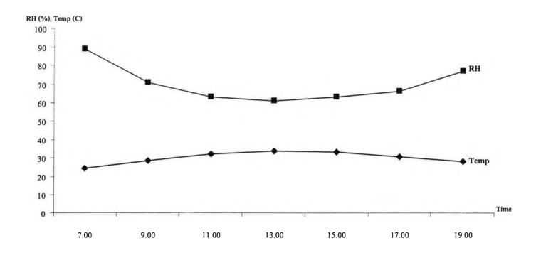
Figure 3. Temperature and relative humidity of NEVAP between 0700 to 1900 h
