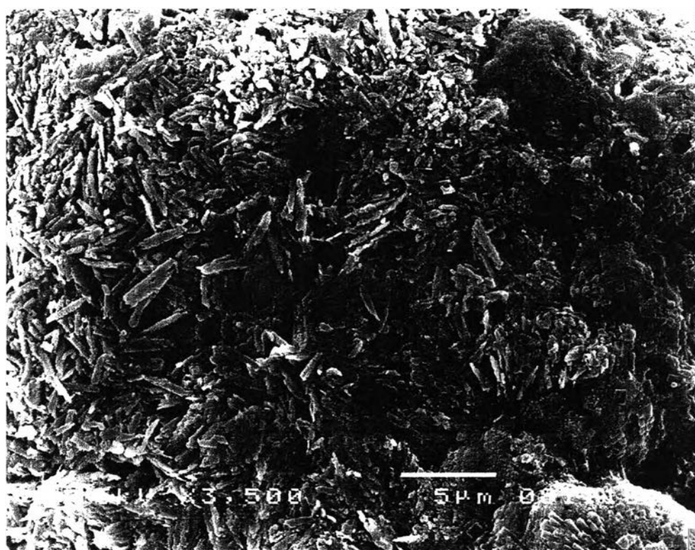
Figure 5.30 Scanning electron micrograph of the coated admicelled rubber (with 200 mM PTh) by using electrochemical method; magnification 1,500/15 kV
