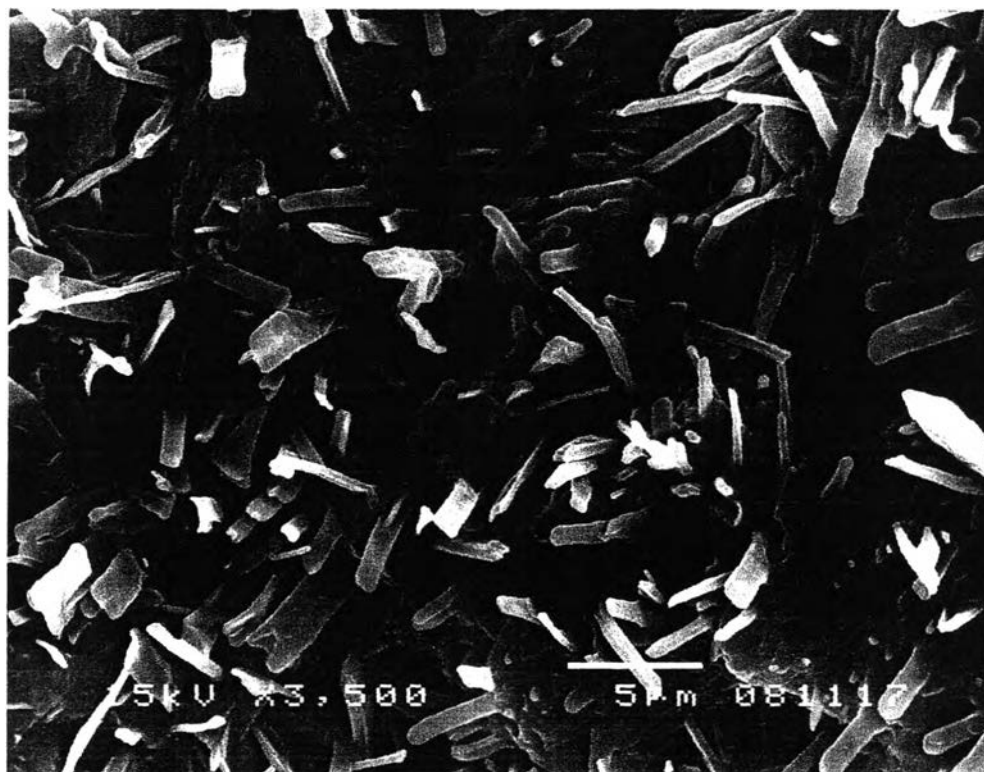
Figure 5.27 Scanning electron micrograph of the coated admicelled rubber (with 20 mM PTh) by using electrochemical method; magnification 1,500/15 kV.
