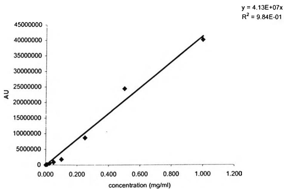
Figure 4.77 Standard curve of Daidzein, AU at 254 nm
