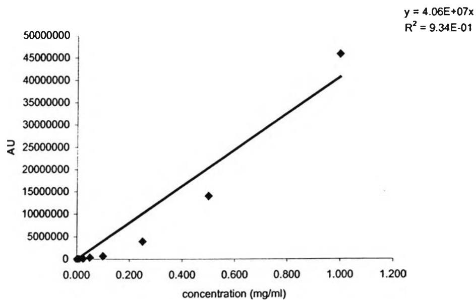
Figure 4.76 Standard curve of Genistin, AU at 254 nm
