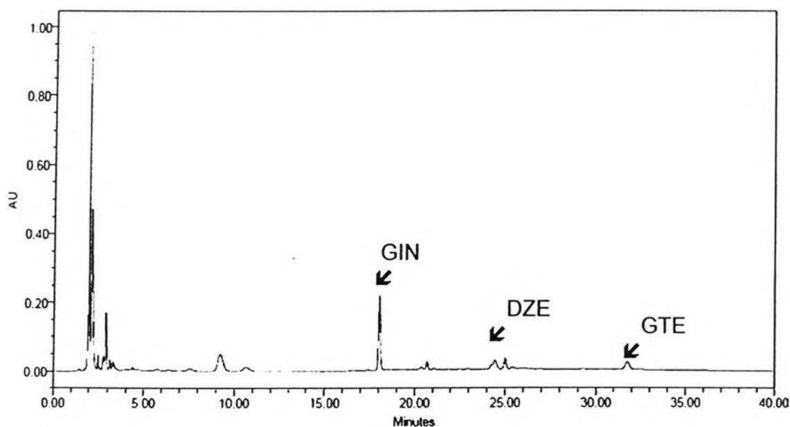
**Figure 4.81** The chromatograms from HPLC analysis of methanol of rat food were compared with standard puerarin (PUE), daidzin (DIN), genistin (GIN), daidzein (DZE) and genistein (GTE).
