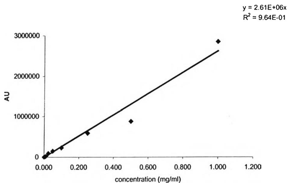
Figure 4.74 Standard curve of Puerarin, AU at 254 nm
