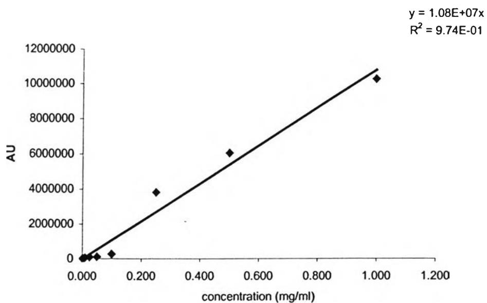
Figure 4.75 Standard curve of Daidzin, AU at 254 nm
