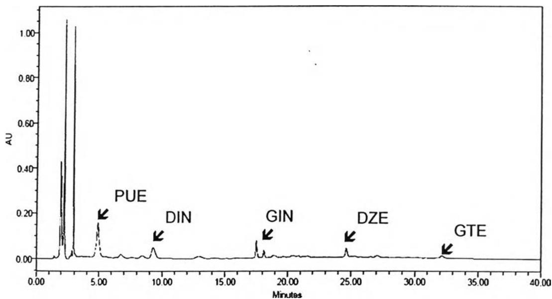
**Figure 4.79** The chromatograms from HPLC analysis of methanol of *P. mirifica* was compared with standard puerarin (PUE), daidzin (DIN), genistin (GIN), daidzein (DZE) and genistein (GTE).
