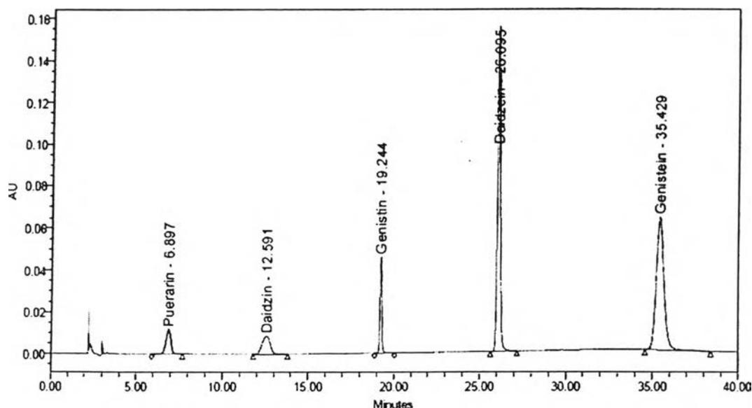
**Figure 4.73** The chromatograms of standard puerarin, daidzin, genistin, daidzein and genistein. Symmetry  $C_{18}$  reversed column was used to separate the aglycones and their glucuronide products. The elution and gradient conditions were described in the method.
