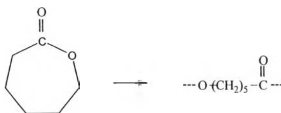
Figure 2.1 The reaction of ring opening polymerization of \epsilon -caprolactone rings.
