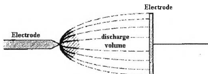
Figure 2.6 The corona discharge-inhomogeneous discharge at atmospheric pressure.
