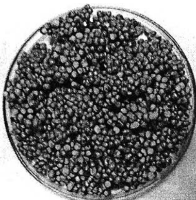
Figure 4.6 Urea fertilizers coated with cardanol-tung oil (A) 6%, (B) 10%, and (C) 15% of cardanol-tung oil.
