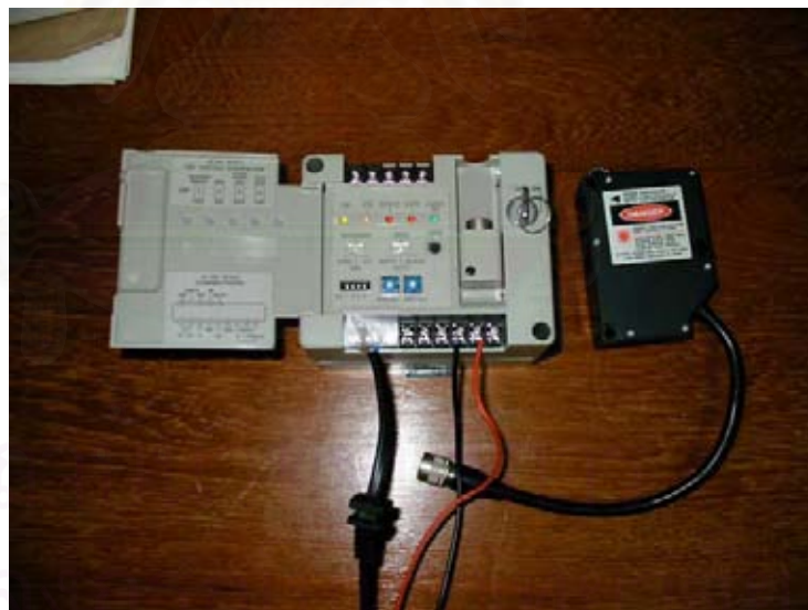
Fig. 3.5 KEYENCE laser displacement system
