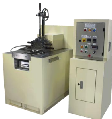
Figure 3.7 CHAREONTUT MX500-D75L90 internal mixer
