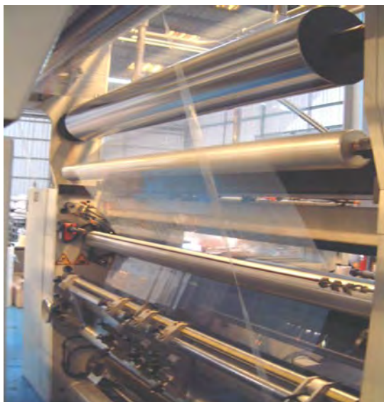
Figure 3.5 Edge trimming before winding
