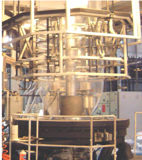
Figure 3.4 External air ring and internal bubble cooling (IBC)
