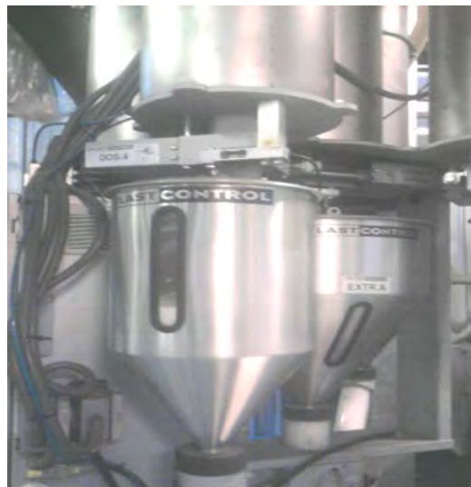
Figure 2.7 Hopper of a blown film extrusion machine
