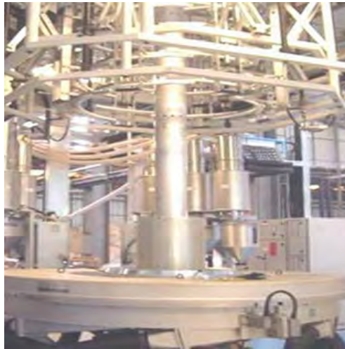
Figure 2.13 Internal bubble cooling (IBC)
