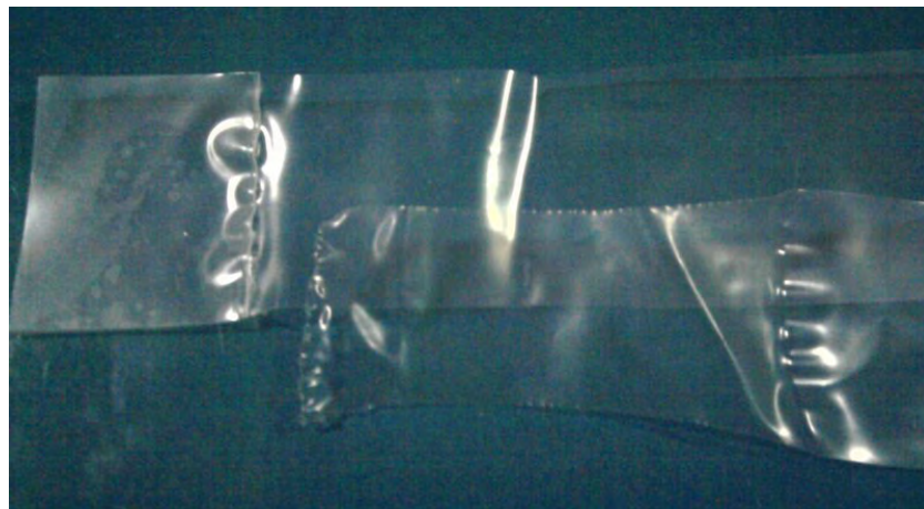
Figure 4.10 Specimen of LDPE/LDPE-re-LDPE/LDPE film after seal strength measurement
