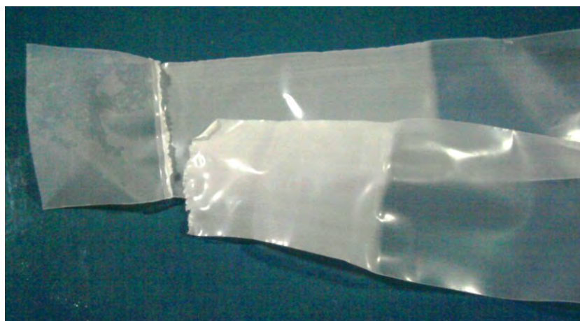
Figure 4.38 Specimen of LDPE/re-LDPE-CaCO 3 /LDPE film after seal strength measurement
