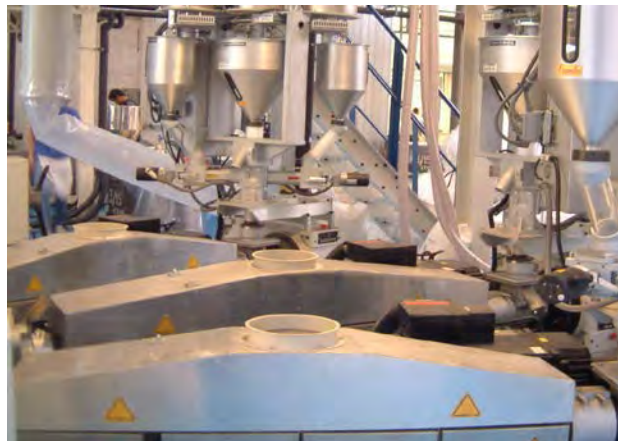
Figure 3.3 Three barrels of co-extrusion machine
