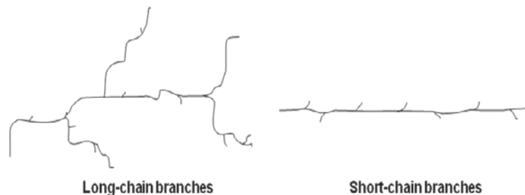
Figure 2.2 PE chains containing different type of branch
