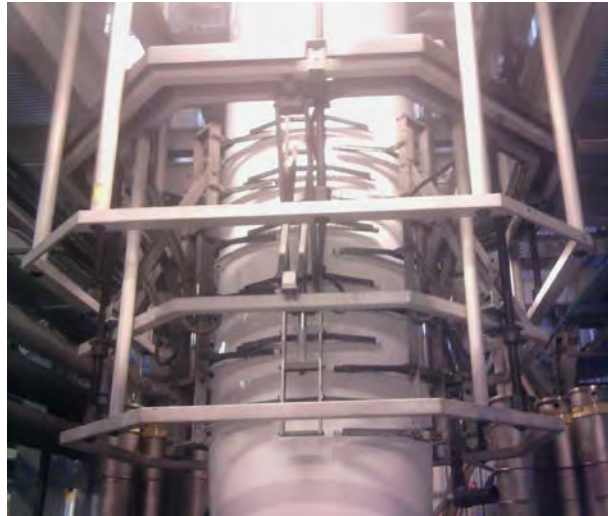
Figure 2.14 A bubble stabilizing cage with Teflon-coated rollers
