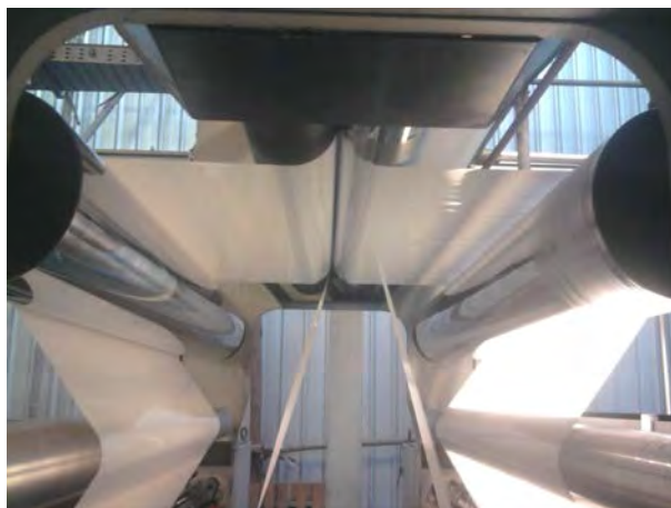
Figure 2.16 A pair of nip rolls with a rubber-covered contact roll
