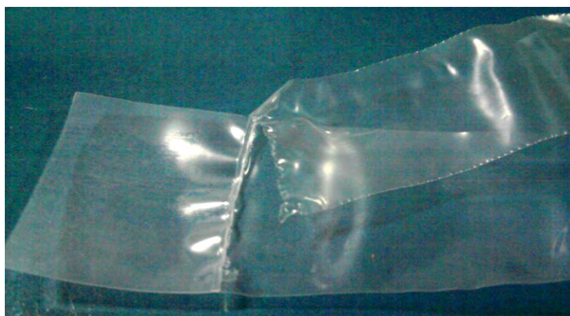
Figure 4.19 Specimen of LDPE/re-LDPE-MDPE/LDPE film after seal strength measurement
