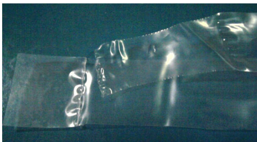
Figure 4.28 Specimen of LDPE-LLDPE/re-LDPE-MDPE/LDPE-LLDPE film after seal strength measurement
