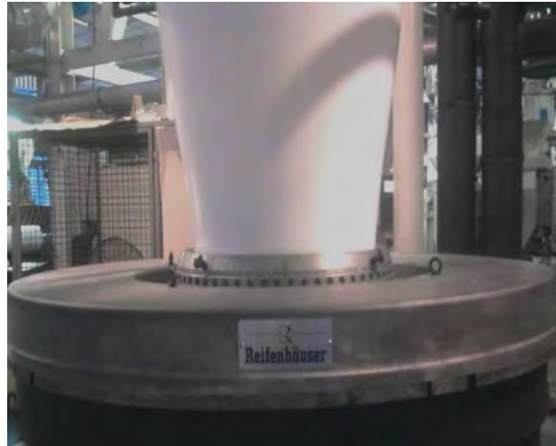
Figure 2.11 A blown film air ring
