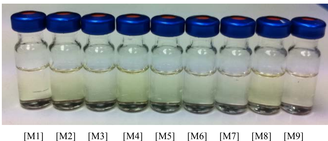
Figure 4.5 Color of blank onion extracts based on different combinations of d-SPE sorbents.
