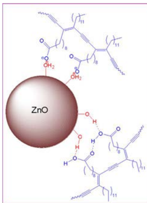
Fig. 2.28 Illustration of hydrogen bonding and ionic interaction between -\text{COOH} and -\text{COO}^- groups of PDA and \text{Zn-OH} and \text{Zn-OH}_2^+ groups at the surface of ZnO nanoparticles [22]
