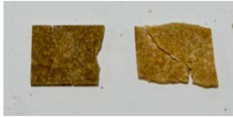
Figure 4.30 Appearance of 5 wt.% MCC/PLA composites (left) untreated MCC and (right) APS treated MCC at 45 days of biodegradation.
