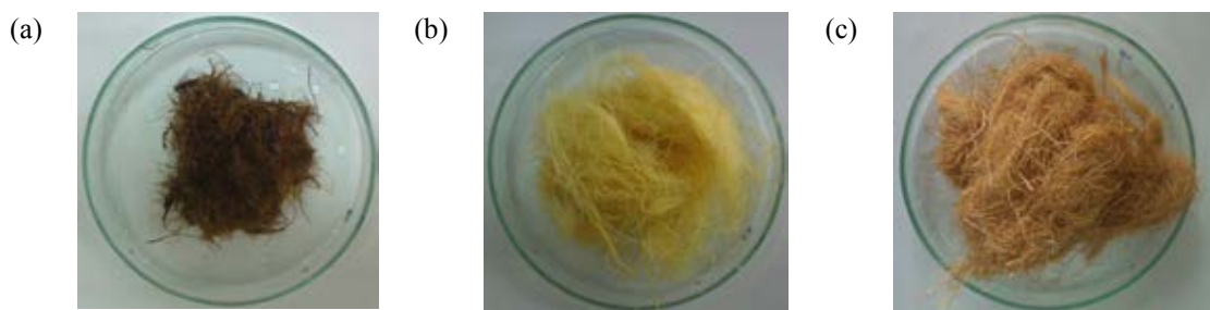
Figure 4.1 Appearance of coir after (a) delignification (b) bleaching (c) hydrolysis
