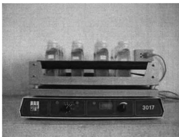
Figure 3.3 The experimental apparatus for the study nickel adsorption with HFO
