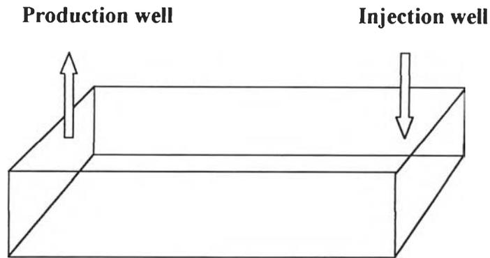
Figure 4.1: Reservoir model configuration.
