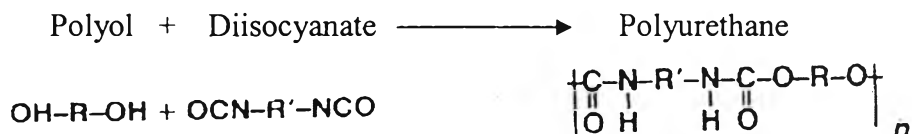
Figure 3.7.2 Polyurethane addition reaction
