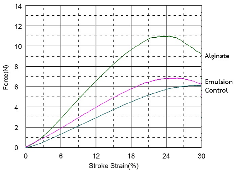
Figure 4F Compression test of coated pitahaya with different coatings compared to control (uncoated) at day 12
