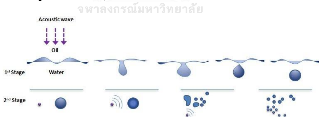
Figure 3 Droplet formation of ultrasound emulsification (Manickam, 2013)
