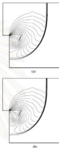
Fig. 3 Diffraction of a Mach 2 shock over a 90^\circ corner: (a) RoeVL; and (b) RoeVLPA.
