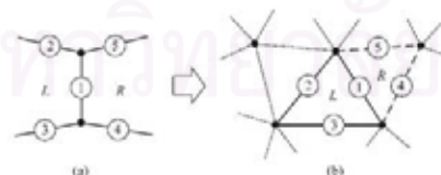
FIGURE 1 Cell interfaces of (a) structured uniform mesh and (b) unstructured triangular mesh.
