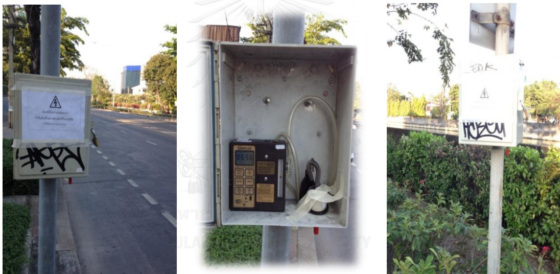
Personal air pump connected to PMI setting at sampling site
