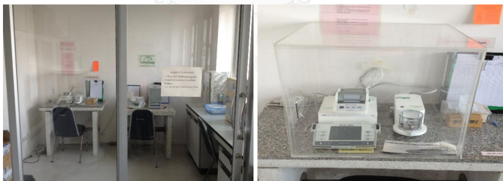
Figure 3.10 Digital ultra-microbalance (METTLER UMX 2) accuracy of 0.001 mg was used to weight the filters before and after particulate matter sampling.
