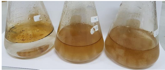
Group A, individually immobilized the bacteria then pooled together with 1:1 AQ weight ratio
