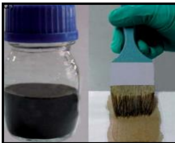
Figure 18 Brush-coating of the graphene oxide ink on cotton cloth [11].
