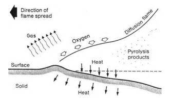
A further factor which determines the extent of flame spread is the heat of combustion of the polymer. The heats of combustion of various polymers are compared with those of cotton and cellulose in Table 2-3
