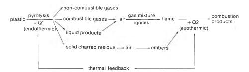
Three stages are necessary to initiate the actual combustion process: heating, decomposition and ignition of the polymer.
