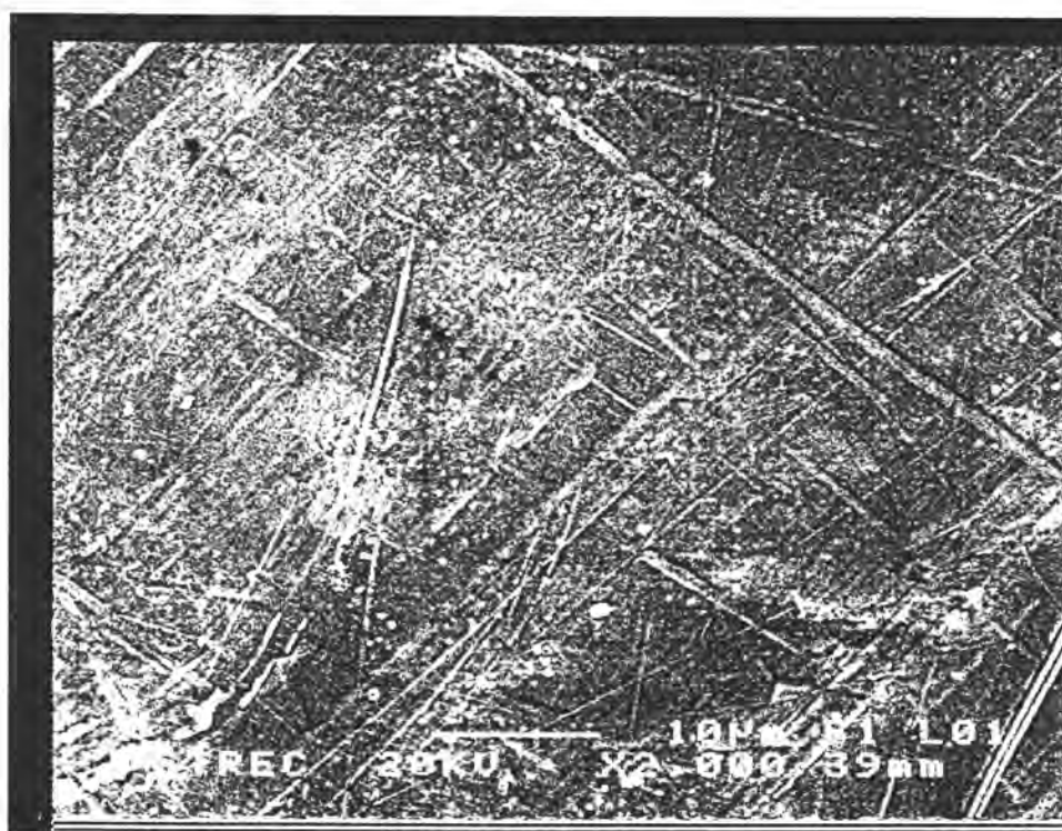
Figure 4-15 Scanning electron micrograph of HIPS resin.
