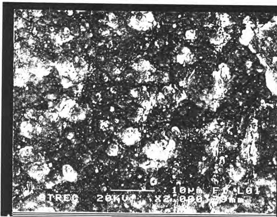
Figure 4-17 Scanning electron micrograph of commercial HIPS resin (ATO CHEM).
