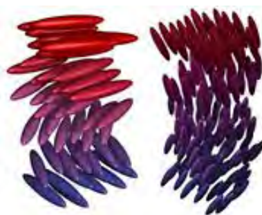
Figure 2.18: Schematic of mesogen ordering in chiral liquid crystal phases.
