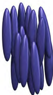
Figure 2.17: Schematic of mesogen ordering in a nematic phase.
