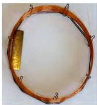
Figure 2.11 Packed column of gas chromatography (GC) (Piantanida et al. , 2014).
