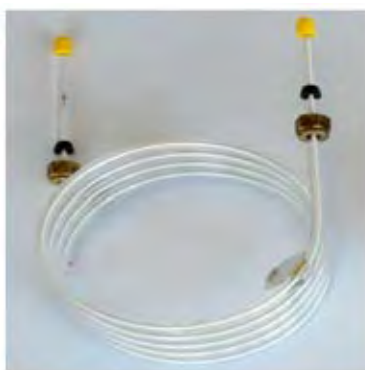
Figure 2.11 Packed column of gas chromatography (GC) (Piantanida et al. , 2014).
