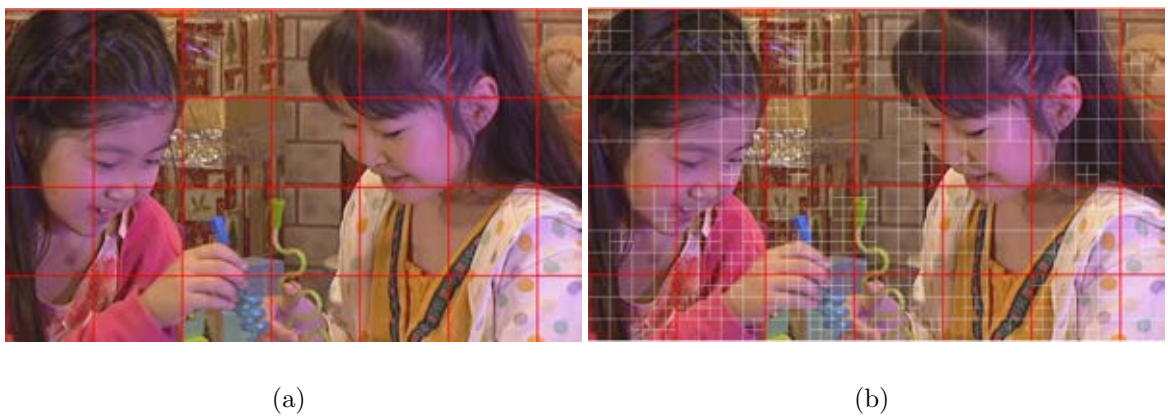
Figure 2.9: Quadtree partitioning of a CTU into CU based on recursive RD cost comparison. (a) Subdivision into 64×64 CTUs. (b) Coding quadtree with CUs.
