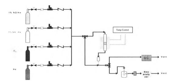
**Figure 3.1** Schematic representation of SCR of NO with NH<sub>3</sub> process flow diagram (adapted from Rochanutama, 2003).
