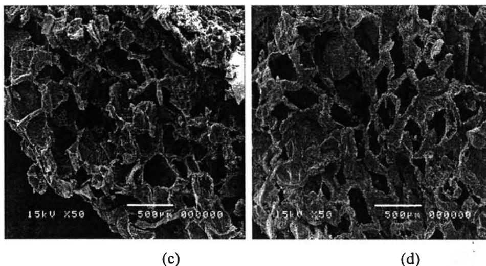
**Figure 5.1** SEM images illustrate microstructure of the scaffolds on the surface: (a) PCL, (b) HAp-PCL and on the cross-sections : (c) PCL, (d) HAp-PCL.
