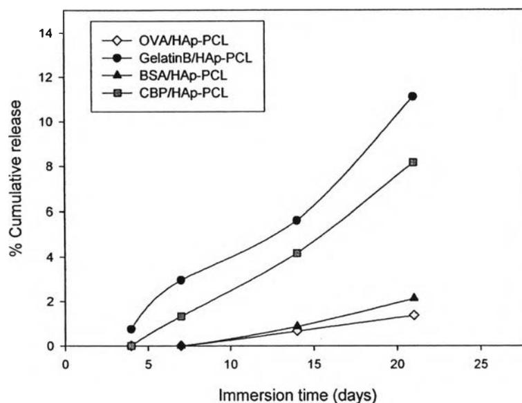
**Figure 5.3** Release profile from protein-loaded HAp-PCL scaffold in 10 % MEM.
