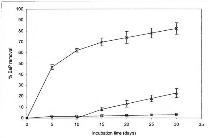
Figure 5.1 Biodegradation of 100-ppm BaP of the fungal isolate in liquid medium. Loss of BaP from auto-degradation ( $\Delta$ ); Loss of BaP from adsorption ( $\square$ ); and BaP Biodegradation (x). (Mean of three replications  $\pm$  S.D.)
