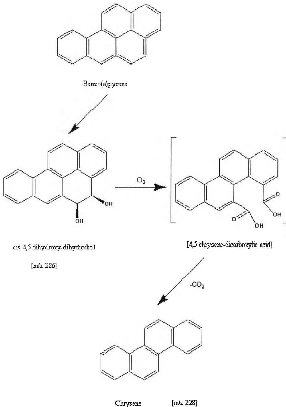
Figure 5.4.2 The oxidation of BaP to chrysene via cis 4, 5-dihydroxy 4,5 dihydrodiol BaP and dicarboxylic acid chrysene generally found in bacteria *Mycobacterium* sp. RJGII-135. Compound in bracket was not detected.
