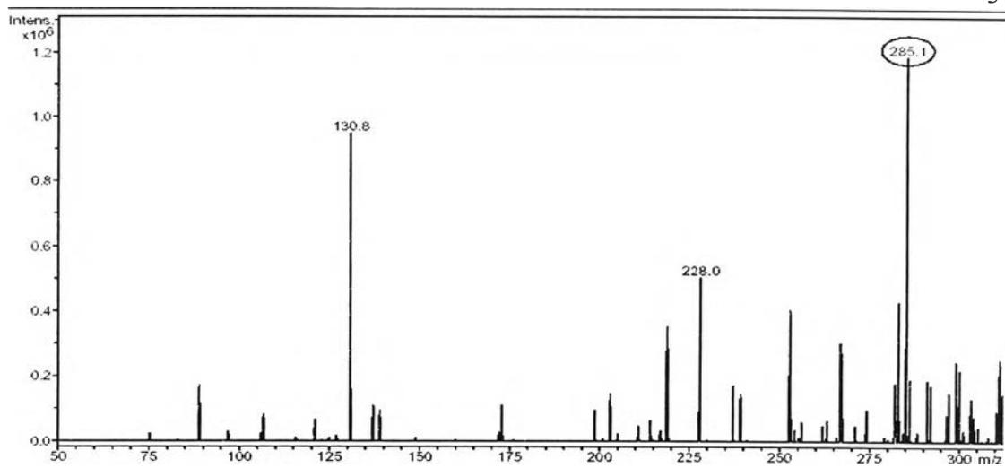
Figure 5.3.1 Mass spectrum of the BaP intermediate obtained at the end of incubation period (30days) from the extra-cellular fraction of *Aspergillus niger* N003 grown in 100 ppm BaP. A molecular ion at MH<sup>+</sup> 285 indicated in circle represents dihydroxy-dihydrodiol of BaP.
