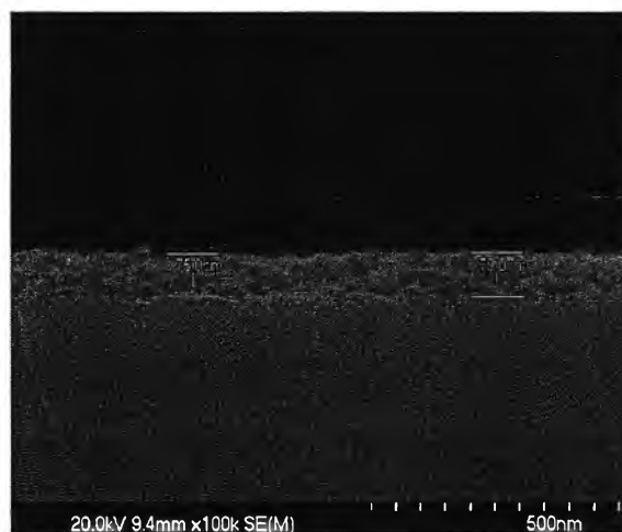
Figure 5.10 Cross section of FESEM image of ZnO coating film prepared from 0.50 M zinc acetate concentration with the withdrawal speeds of 9.0 cm/min
