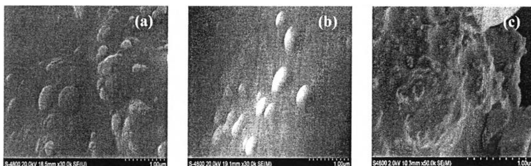
Figure 5.3 The SEM micrographs of (a) PMPS-ad-NR 50 mM, (b) PMPS-ad-NR 100 mM and (c) PMPS-ad-NR 200 mM.
