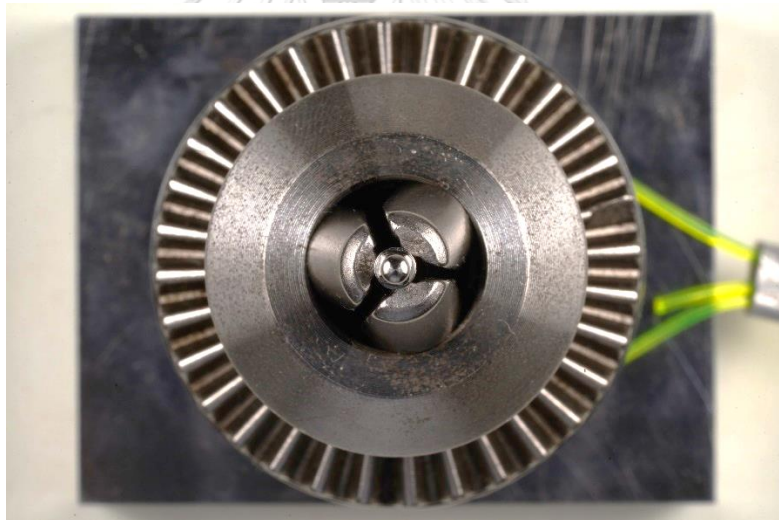
Figure 5 Mini-implant abutment mounted in the testing apparatus
