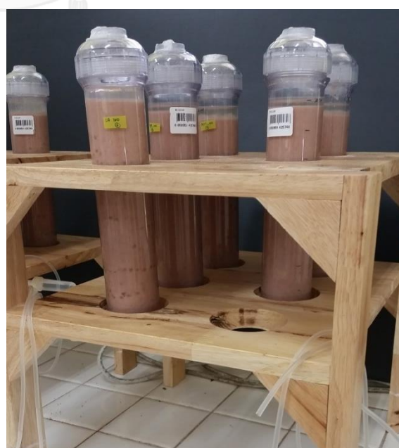
Figure 6.1 Profenofos biodegradation in column experiment in free and immobilized cells at different concentration of profenofos
