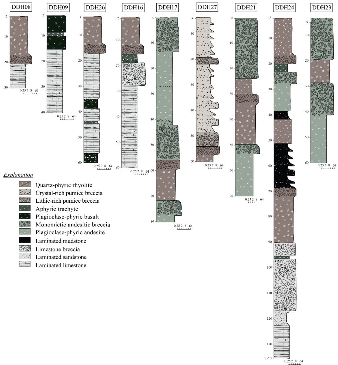
Fig. 3.2 Simplify graphic log of selected drill holes, in geographic order from northernmost at the left to the southernmost at the right. See Fig. 3.1C for location of drill holes.
