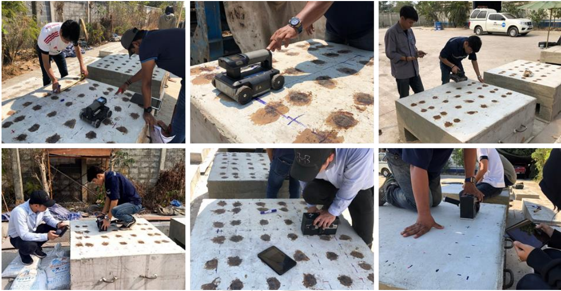
Figure 27. Line-scan testing over the hardening period was performed by GPR and UPE methods.
