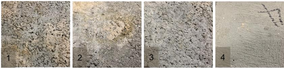
Figure 25. Four unconsolidated concretes illustrate the difference of void and concrete ratio by naked eyes.
