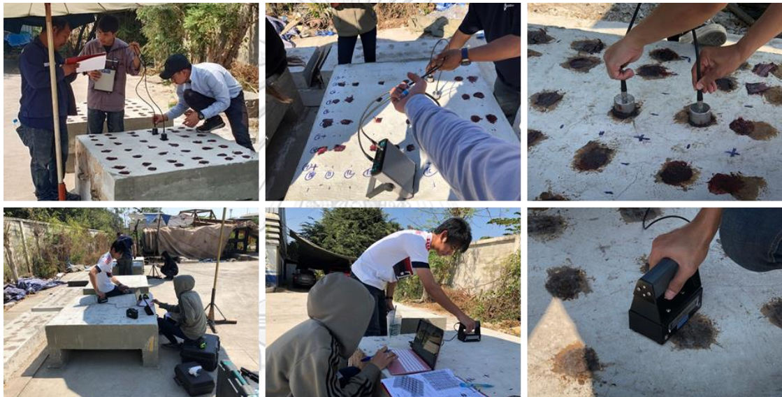
Figure 33. Line-scan testing over the hardening period was performed by IE and UPV methods.
