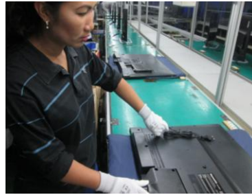
Figure 5.12 Power wire installation
