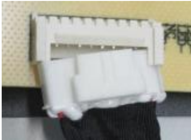
Figure 4.9: Inappropriate installation of wire in TV panel
