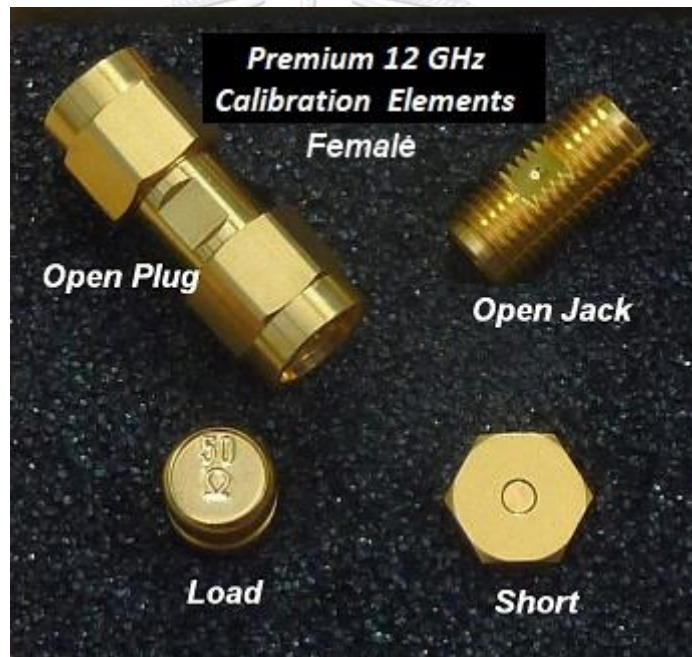
Figure 4.1 Premium FEMALE SMA SOL 4 pcs Calibration Kit of 12 GHz Parts.
