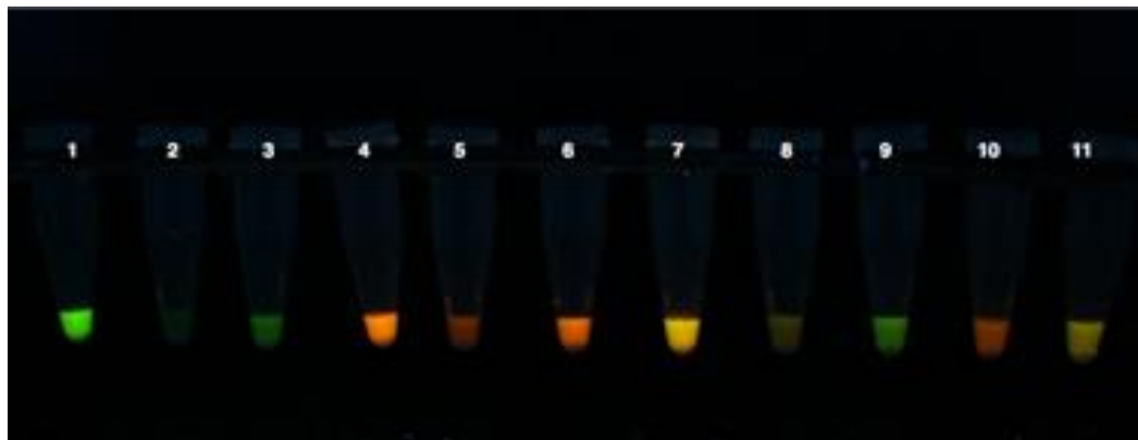
Figure 3.16 Dual color naked-eyed detection; tube1 :FluK5, tube2 :FluK5 + GO, tube3 :FluK5 + GO + dcomFlu, tube4 :TMR-O-K4, tube5 :TMR-O-K4 + GO, tube6 :TMR-O-K4 + GO + dcomTMR, tube7 :mixedPNA, tube8 :mixedPNA + GO, tube9 :mixedPNA + GO + dcomFlu, tube10 :mixedPNA + GO + dcomTMR, tube11 :mixedPNA + GO + dcomFlu + dcomTMR Conditions: [PNA] = 10 \mu M, [DNA] = 12 \mu M, [GO] = 50 \mu g/mL in 10 mM Tris-HCl pH 7.4; FluK5 :Flu-GTAGATCACT-KKKKKNH 2 , TMR-O-K4 :TMR-O-CTAAATTCAGA-KKKKKNH 2 , dcomFlu :5'-AGTGATCTAC-3', dcomTMR :5'-TCTGAATTTAG-3'
