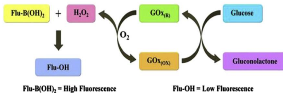
Scheme 3.2 The GOx enzymatic mechanism for detection of glucose using boronic derivative as fluorescence sensor [16].
