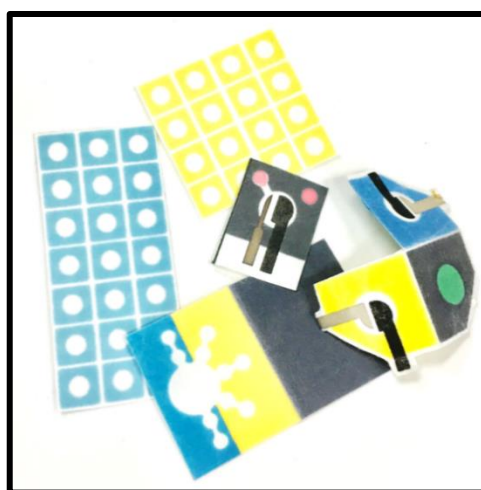
Figure 2.1 Photo of PAD fabricated by wax-printing methods
