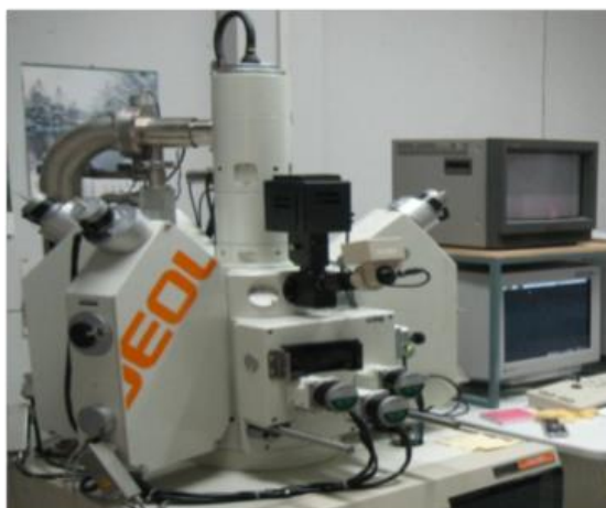
Figure 3.8 JEOL JXA-8100 model of EPMA spectrometer based at Department of Geology, Faculty of Science, Chulalongkorn University.
