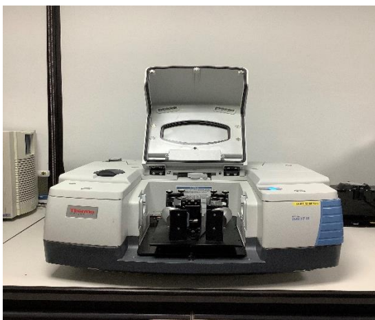
Figure 3.6 Nicolet iS50 FTIR spectrometer based at the Gemological Testing Laboratory, the Gem and Jewelry Institute of Thailand (Public Organization) engaged for this study project.
