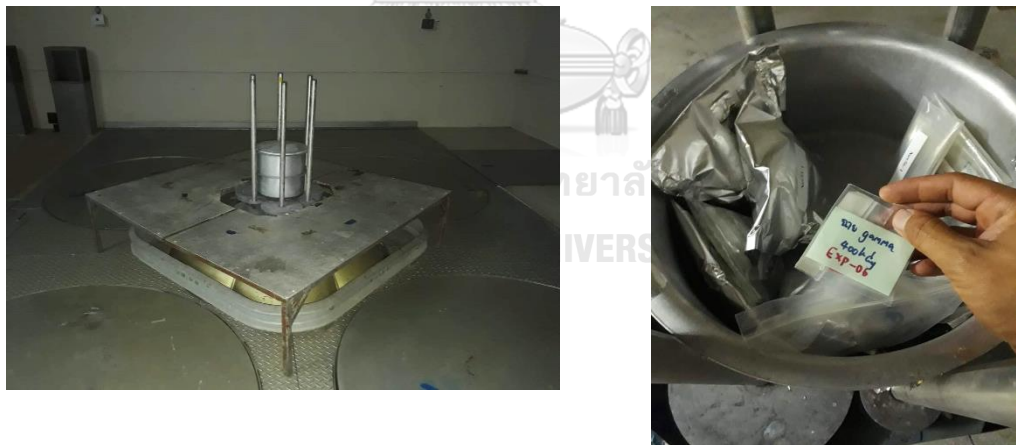
Figure 3.15 (left) six pieces of cobalt-60 sources were used as gamma radiation source. (right) sample preparation for gamma irradiation (Photo by T. Utapong).
