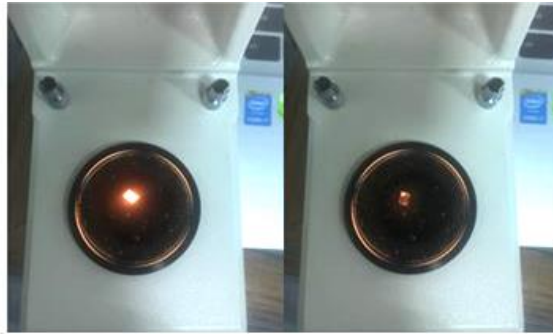
Figure 3.2 Optic character of tourmaline samples under polariscope displaying alternate dark and bright during rotation of the sample every 45 degree.
