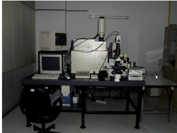
Figure 3.7 Raman spectrometer, model T64000 JOBIN YVON HORIBA based at Department of Physics and Materials Science, Chiangmai University.
