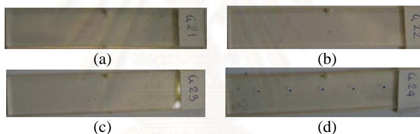
Figure 4.10 Sheet appearance of ST-MMA copolymer sheet (ST/MMA = 20/80) with (a) 1 (b) 2 (c) 3 and (d) 4 wt% grafted natural rubber.
