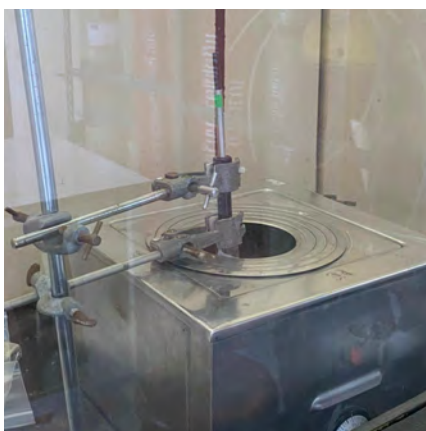
Figure 6. Hot water bath set up where the vial is heated for HS-SPME.
