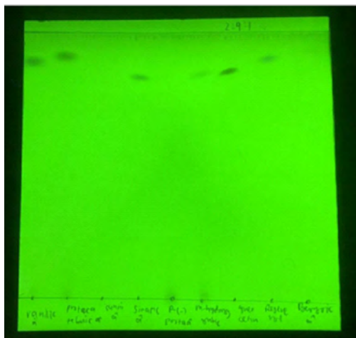
Figure 10. 1000 ppm Standard solutions after performing thin layer chromatography in a total of 9 standards.
