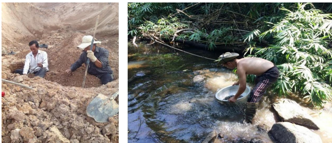
Figure 2.3 Artisanal miners used crowbars and shovels to remove topsoil and dig through the gem-bearing layer in Binh Thuan gem field (left). Gem-bearing gravels were washed and sieved along the local stream in Dak Nong gem field (right). Photos by Doan Thi Anh Vu.
