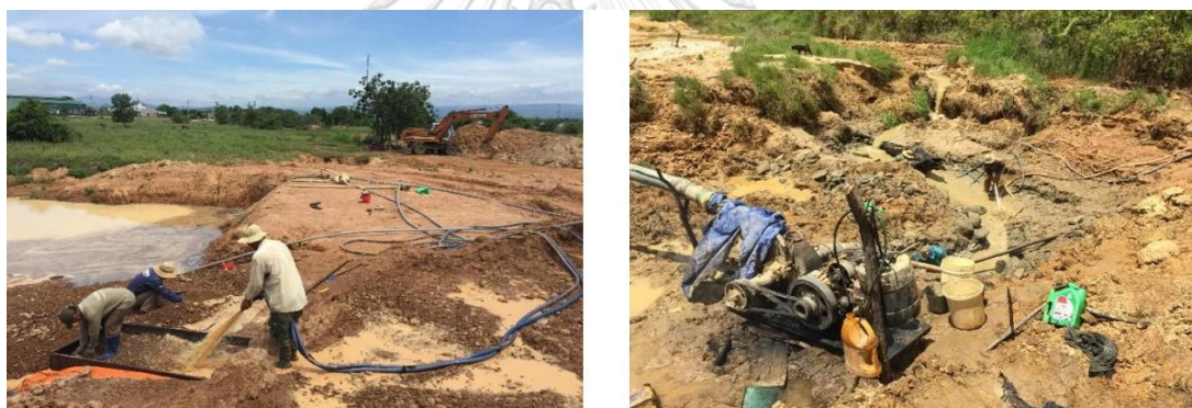
Figure 2.4 Backhoe was used in a machinery mine to remove topsoil and reach the gem-bearing gravel layers prior to washing and dressing using water pump in Binh Thuan gem field (left) and Krong Nang gem field (right). Photos by Doan Thi Anh Vu.
