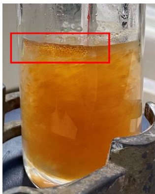
Figure 18 Partial the resin was edged of the reactor during transesterification
