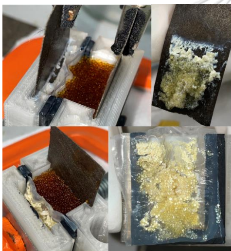
Figure 26 Some solid in anode compartment during electrochemical regeneration
