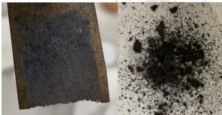
Figure 12 The electrode of anode was oxidized and deposited with carbon
