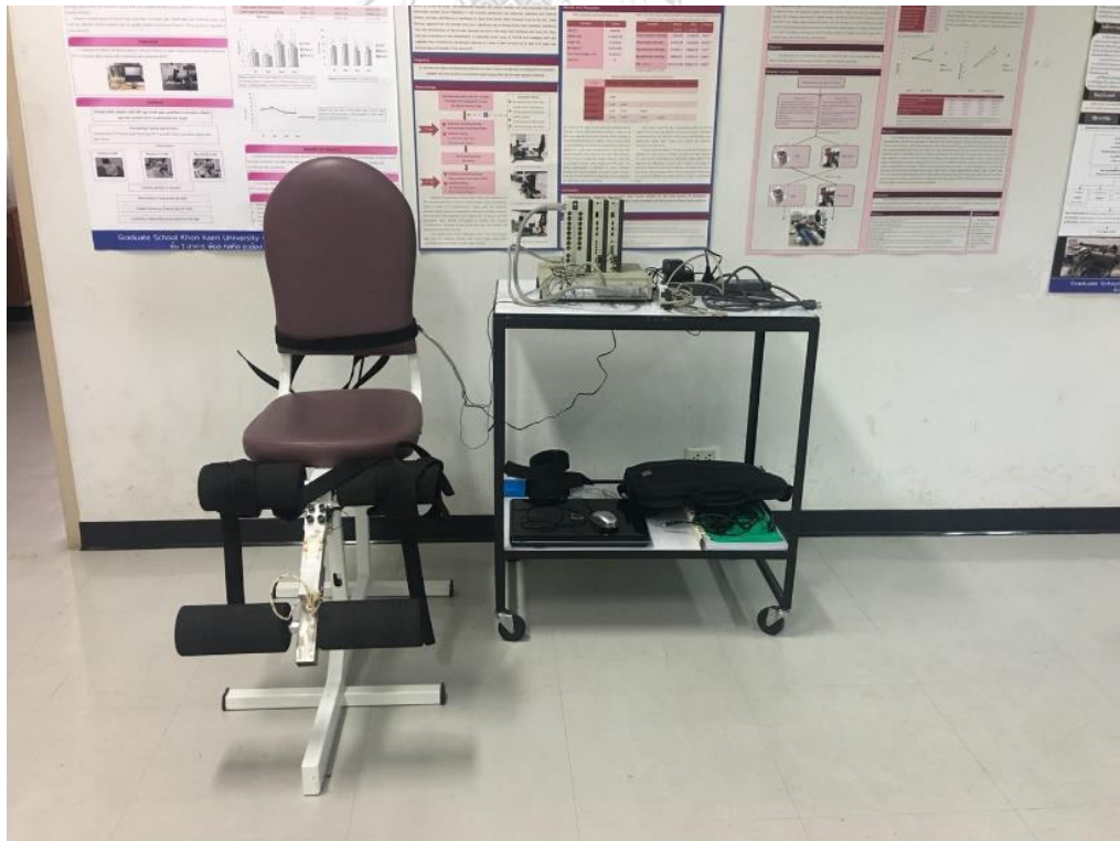
Figure 32 A modified isometric dynamometer
