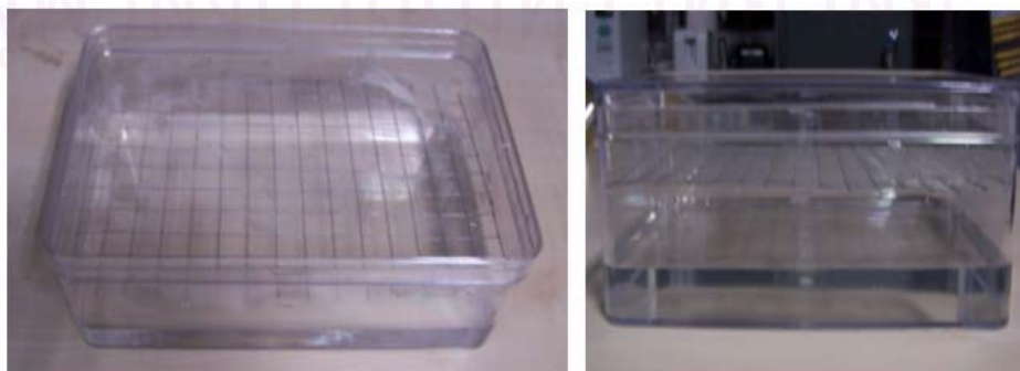
Figure 4.2: Plastic box in moisture absorption test.
