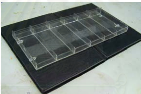
Figure 4.1: Polystyrene mold for MC film casting.
