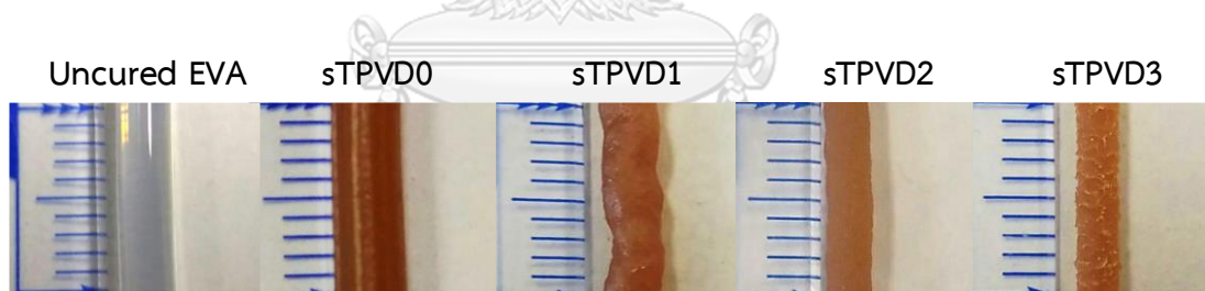
Figure 4.12 Extruded strands of uncured EVA and EVA/NR TPVs at 190 °C
