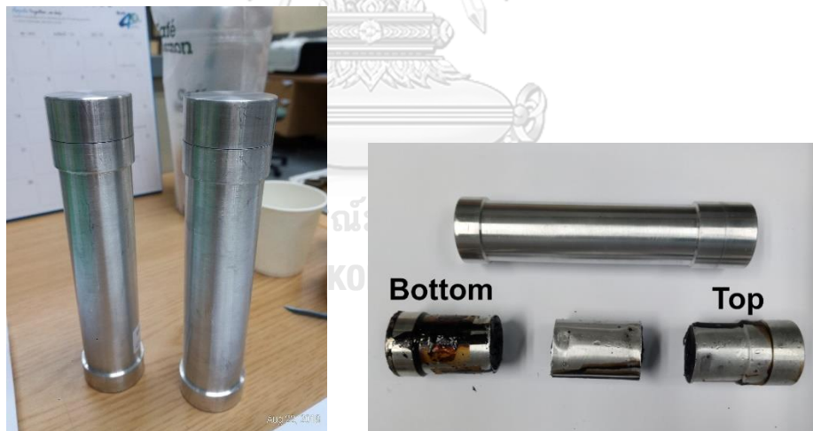
Figure 3.9 Appearance of aluminum tube (left) and its three sections: Top, Middle, and Bottom (right)
