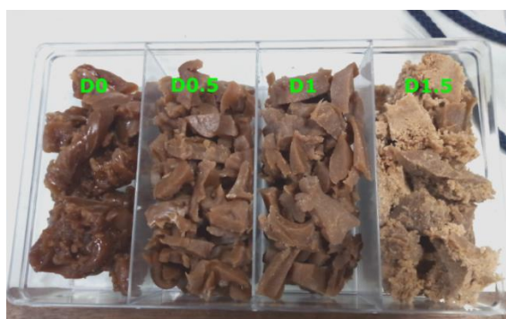
Figure 5.2 Appearances of EVA/NR thermoplastic vulcanizates at various DCP contents
