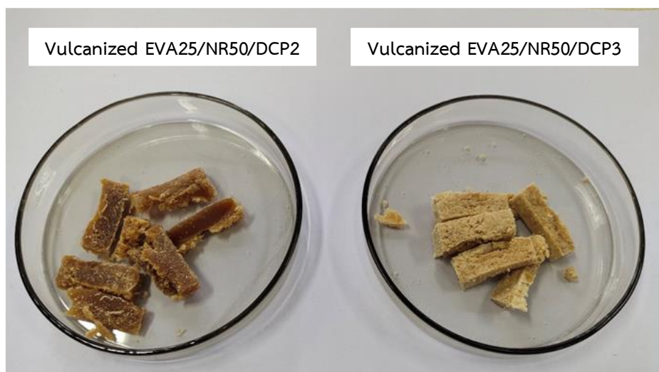
Figure B.1 Vulcanized sample from the internal mixer of 30 cm 3 (left) EVA25/NR50/DCP2 (right) EVA25/NR50/DCP3
