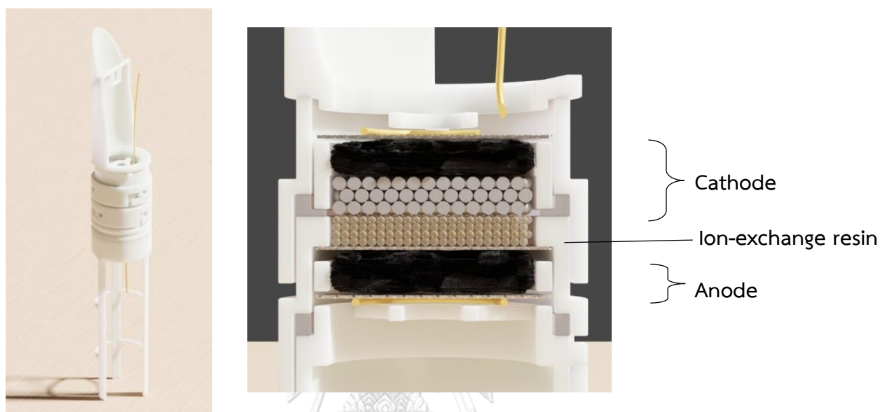
Fig. 10 Electrochemical CO 2 RR cell configuration
